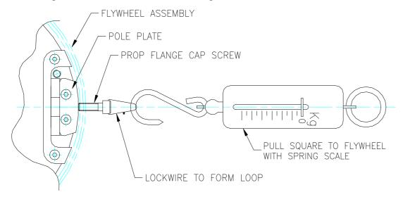
Drawing 9437064/1 MAGNET PULL TEST - FLYWHEEL
