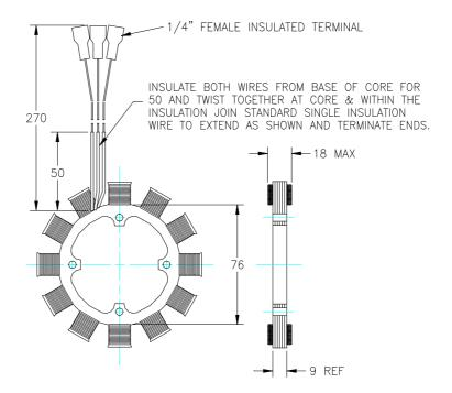
Drawing 4665084/1 ALTERNATOR CORE ASSEMBLY
