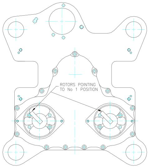
Drawing 9431064/1 REAR PLATE GEAR HOUSING & ROTORS
