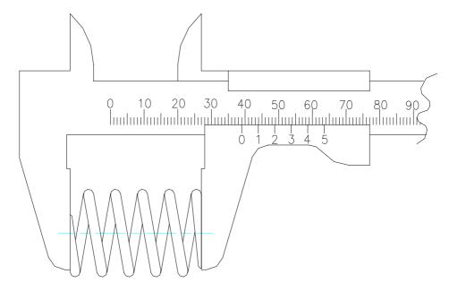
Drawing 9443064/1 VALVE SPRING MEASUREMENT
