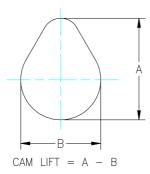
Drawing 9433064/1 CAM LIFT MEASUREMENT
