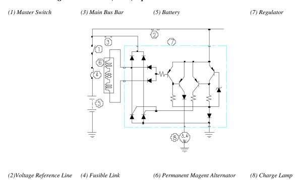
The charging system supplies electrical devices and also charges the battery while the engine runs. It consists of a Permanent Magnet Alternator (PMA) and a Regulator.
