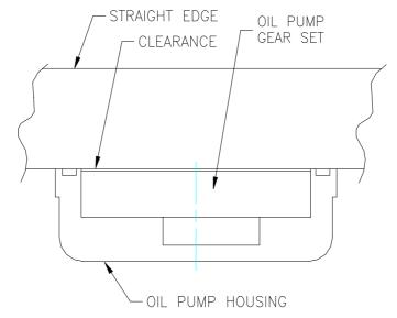
Drawing 9428064/1 OIL PUMP END CLEARANCE
