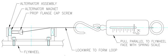
Drawing 9438064/1 MAGNET PULL TEST - ALTERNATIOR
