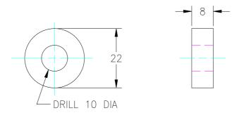
Drawing 9442064/1 SPACER FOR MEASURING CRANKCASE
